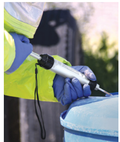
First responder uses RAE Systems colorimetric tubes and hand pump to measure VOC levels inside a barrel.
