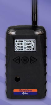
The EchoView Host mini-controller is the cornerstone of RAE Systems' Closed-Loop Wireless Solutions for portable gas monitors. This rugged handheld device can establish a self-contained wireless network with up to eight supported RAE Systems portable monitors and display their readings and alarm status in real time on an easy-to-read screen.
