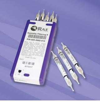
The Humidity Filtering II Tube dries the sample gas entering pumped instruments. It is particularly suited for removing humidity effects on photoionization detectors (PIDs) while making VOC measurements, and typically lasts for about a half hour of continuous readings. The Humidity Filtering II Tube utilizes a solid adsorbent to remove moisture without impacting the detection and measurement of most VOCs.
