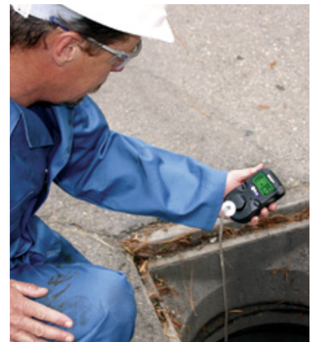
QRAEII Pump being used for a confined space entry
