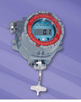
The RAEGuard PID is a permanently mounted (fixed) Photoionization Detector (PID) transmitter that operates from a 9 to 36 VDC power source and provides an analog (4-20 mA) signal output in three fulls-cale ranges of 20 ppm, 100 ppm, or 1,000 ppm isobutylene equivalent. Housed in an explosion-proof enclosure, the RAEGuard PID is equipped with a local digital display of the gas concentration and functional keys for performing calibration.
