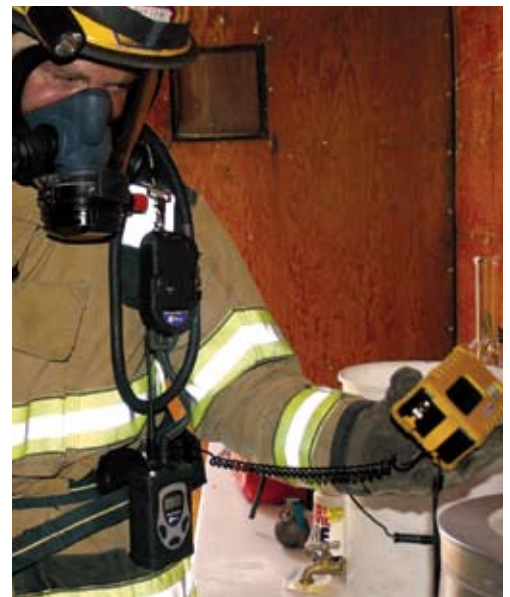
Hazardous Material Response Team member using MultiRAE Plus and GammaRAE II R with RAELink3 Z1
