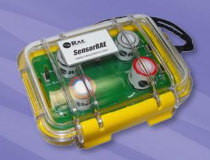
The SensorRAE is a compact waterproof conditioning station that keeps up to four RAE Systems' interchangeable electrochemical (EC) sensors warmed up and ready for immediate installation, calibration, and use in RAE Systems MultiRAE Plus and AreaRAE monitors. The SensorRAE offers users of these monitors the ability to broaden the spectrum of detectable compounds by having four additional EC sensors readily available in addition to the four EC sensors installed in the instrument.
