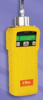
The VRAE is a powerful, pumped, one- to five-gas monitor that protects workers from combustible gases and vapors, toxic gases and oxygen deficiency/enrichment. This versatile instrument can measure concentrations of combustibles either as percentage by volume or as percentage of lower explosive limit (LEL). The VRAE's rechargeable Nickel-Metal-Hydride battery, powerful internal pump and rugged frame make it ideal for confined space entry, leak detection, and site surveys.
