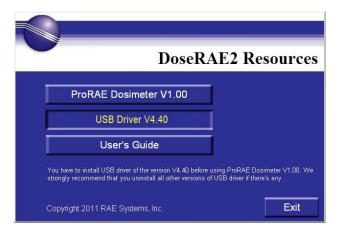
**Important!** If an earlier USB Driver version is installed, it is highly recommended that you uninstall it before installing this version.
