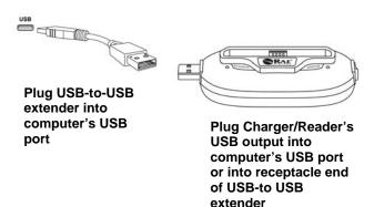
If the computer is on, the Charger/Reader's "Power" LED should glow red when connected to the USB port.
