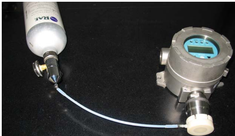
RAEGuard S connected to gas cylinder with a calibration adapter.
